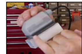
Pressing the Base into the Lid squeezes the silicone into the gaps. Figure 15
